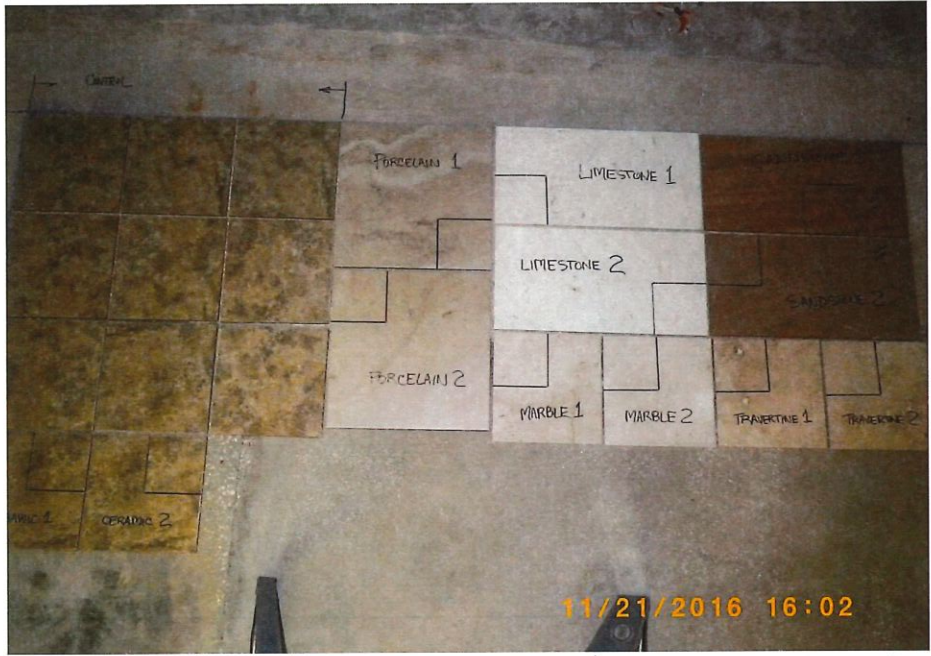
Photo 1: Floor tiles (i.e., ceramic, porcelain, limestone, marble, travertine and sandstone) tap tested for audible character and predominant frequency.
