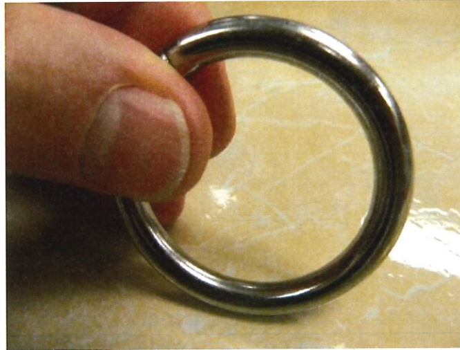
Photo 3: A 2-inch diameter stainless steel ring provided the most distinctive frequencies to distinguish bonded from nonbonded tiles.
